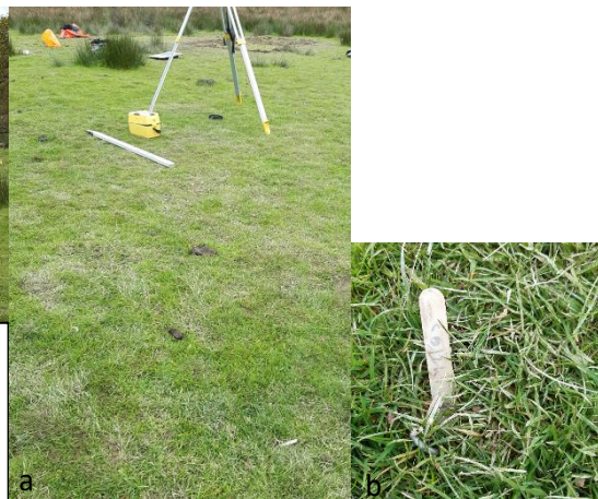
Images 23a-b Dumpy level and close up of TBM (Temporary Bench Mark)
