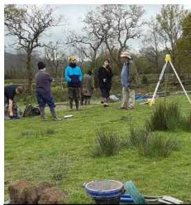
Image 22: Day 2 Using the dumpy level to get the AOD (Above Ordnance Datum)
