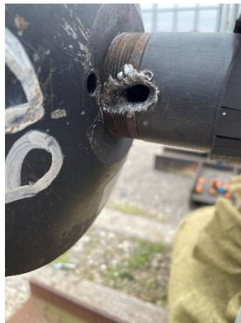
Figure 6 – Blast Gauge 1 Fragmentation Strike
