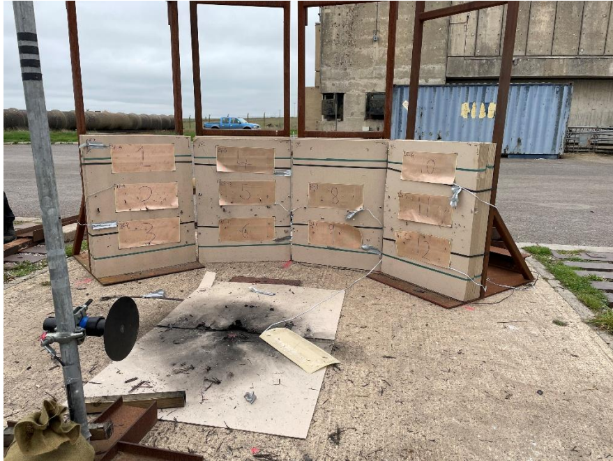
Figure 5 – Post Blast Straw Board Perforation
