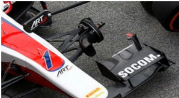
Figure 11 - Dallara GP2/11 Brake Duct (FIA Formula 2, 2017)
