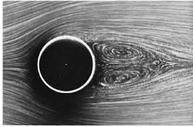
Figure 7 - Wake Formation Behind Cylindrical Object (Wenjun, et al., 2018)
