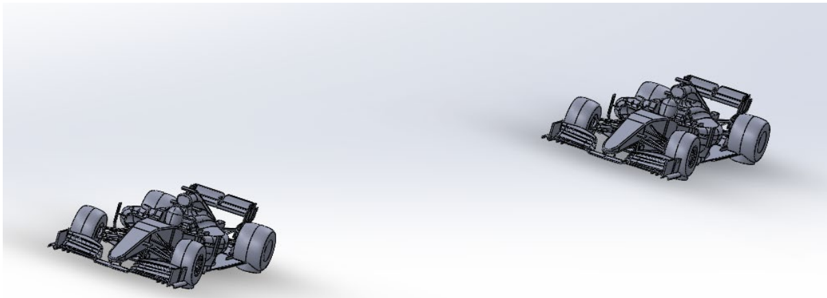
Figure 59 - Following Car CFD Testing Geometry 2019 Spec Cars
