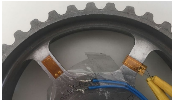
Figure 25 strain gauge setup on pulley spokes
