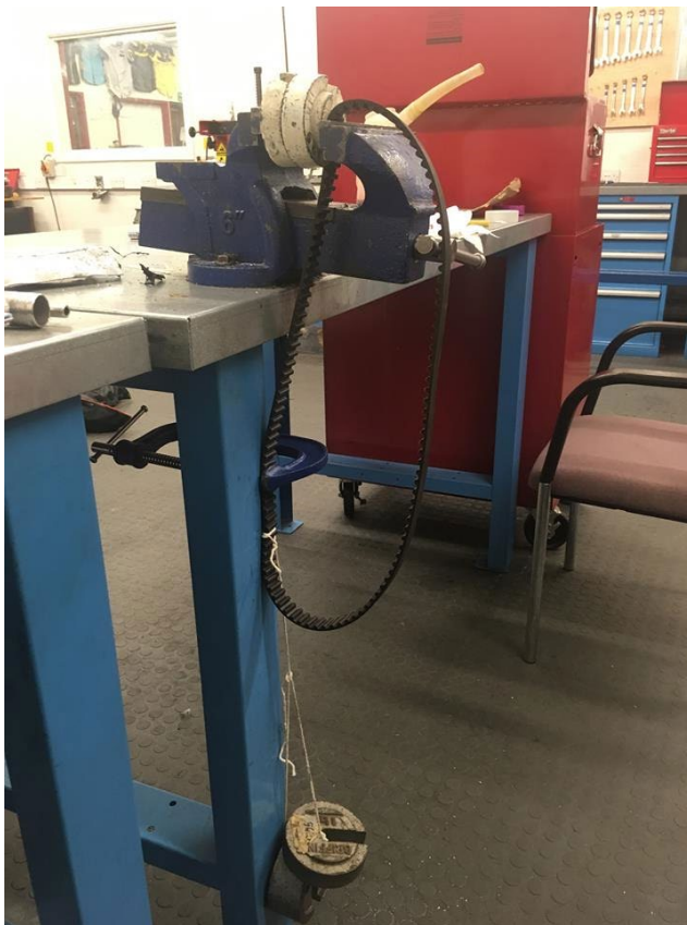
Figure 14 initial cambelt tension experiment setup
