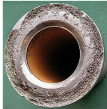
Figure 5: Pitting Corrosion on Flange
