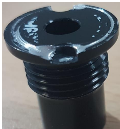
Figure 10 Purposely damaged primary cartridge base
