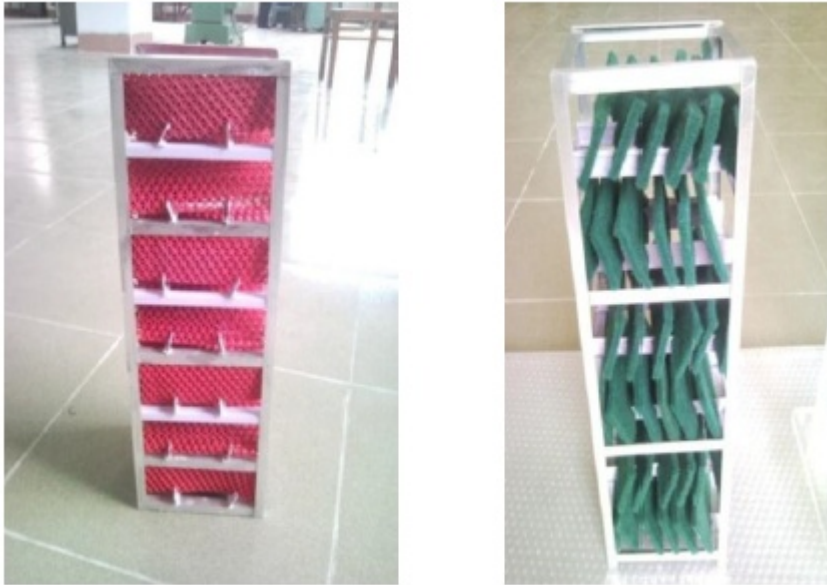
Figure 23: shows different layout for the fins used as evaporative pads (MD.Mahmoud et al,2012)
