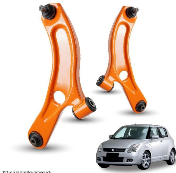
Figure 2 lower arm from Suzuki Swift with fixed ball joint
