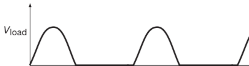
Figure 7 - Single Phase Half Wave Rectifier Voltage Waveform
