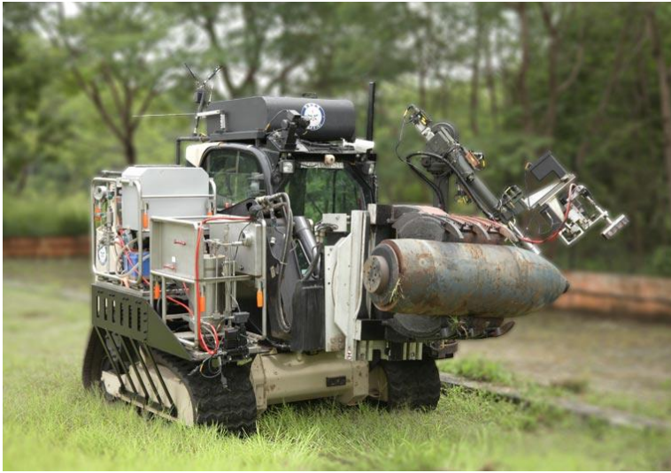
FIGURE 15 - DAKSH UXOR FITTED WITH MACE CUTTING SYSTEM AND SECTIONED DETONATOR EXAMPLE [26]
