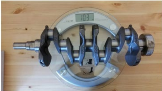
Figure 3-5 4A-GE & EcoBoost crank mass (Evans, 2019)
