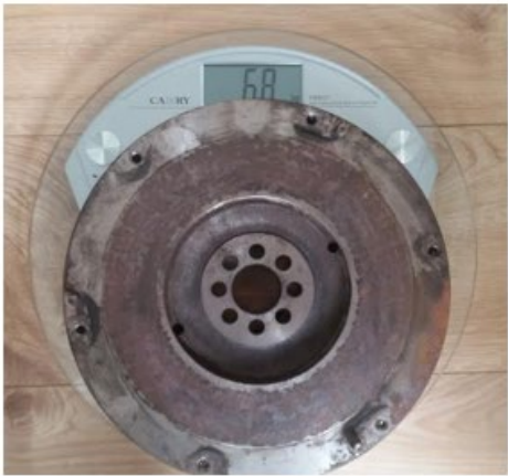
Figure 3-6 4A-GE & EcoBoost Flywheel Mass (Evans, 2019)
