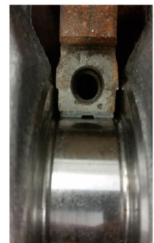
Figure 3-13 Ecoboost crank sitting in 4A-GE Block. notice clearance issue on centre image. image on left shows centre main where thrust washer seats need machining to suit crank
