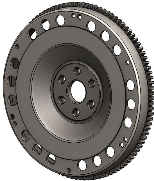
Figure 4-6 New design of flywheel to required dimensions of hybrid 4A-GE see appendix for Engineers drawing (Evans, 2019)
