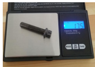
Figure 3-3Bolts mass, notice the 4A-GE uses nut & bolt arrangement. (Evans, 2019)
