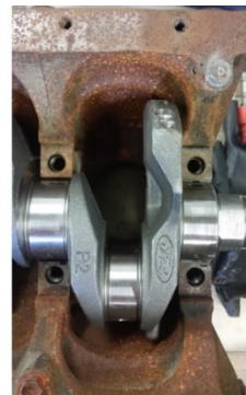
Figure 3-13 Ecoboost crank sitting in 4A-GE Block. notice clearance issue on centre image. image on left shows centre main where thrust washer seats need machining to suit crank
