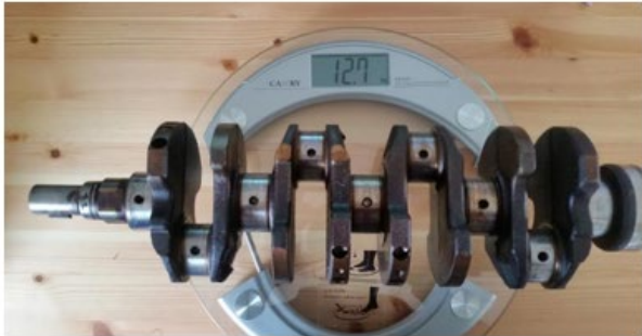
Figure 3-5 4A-GE & EcoBoost crank mass (Evans, 2019)
