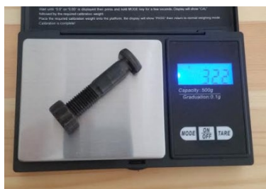
Figure 3-3Bolts mass, notice the 4A-GE uses nut & bolt arrangement. (Evans, 2019)
