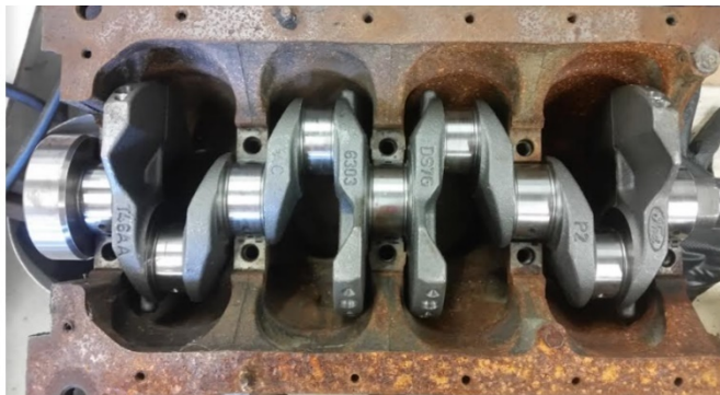
Figure 3-13 Ecoboost crank sitting in 4A-GE Block. notice clearance issue on centre image. image on left shows centre main where thrust washer seats need machining to suit crank
