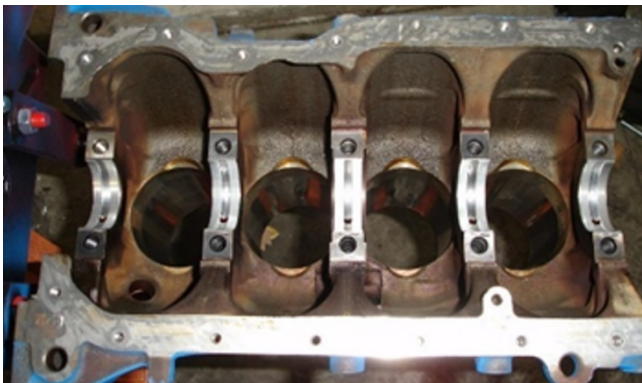
Figure 3-14 7A-FE crankcase, note the machined areas at the base of the bores for the conrods to clear.
