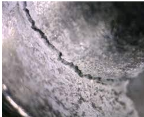
Figure 13: Image showing cracking in the die cast material.
