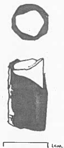
Fig. 8.18 Form of a wooden peg (shaded) preserved by the corrosion products of an iron rivet shank (centre); part of an oak strake adheres on l. side. Gr279. Scale 1:1. Drawn by C. W. Gregson © National Maritime Museum
