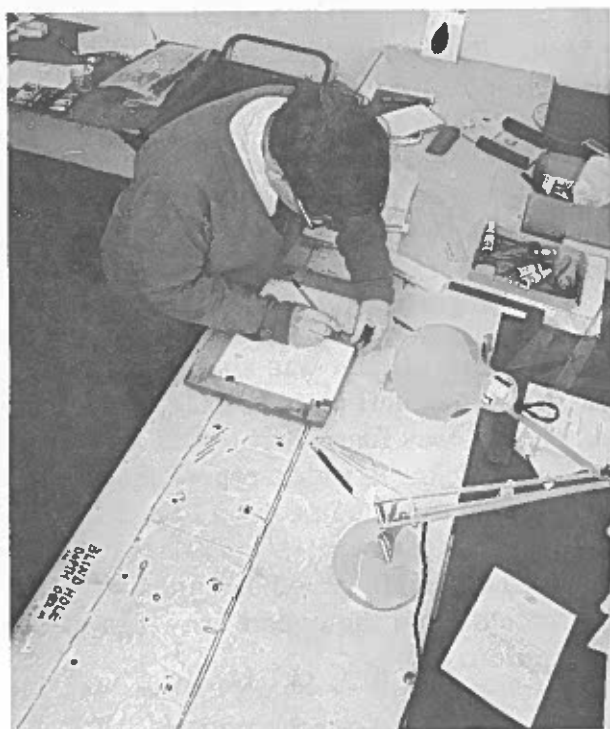
Fig. 2.3.7 Reducing full-scale tracing of a plank to a 1:10 scale drawing © National Maritime Museum
