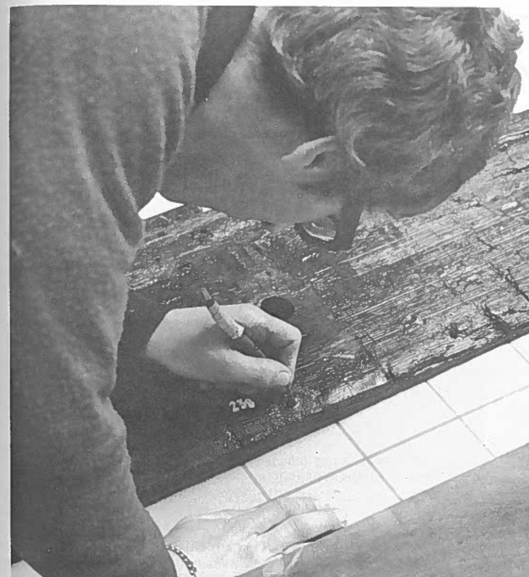
Fig. 8.17 Details of construction, such as wooden pegs inserted in the strake-fastening holes before iron rivets driven in, were revealed by careful cleaning. © National Maritime Museum
