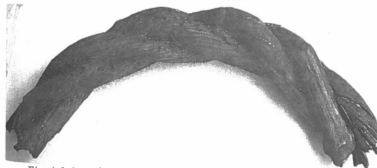
Fig. 1.2.6 Three-strand rope, Gr15 (0.14 m long) from beneath port side. After impregnation with polyethylene glycol it was strong enough to handle. The structure of vegetable fibres was too incoherent for identification © National Maritime Museum
