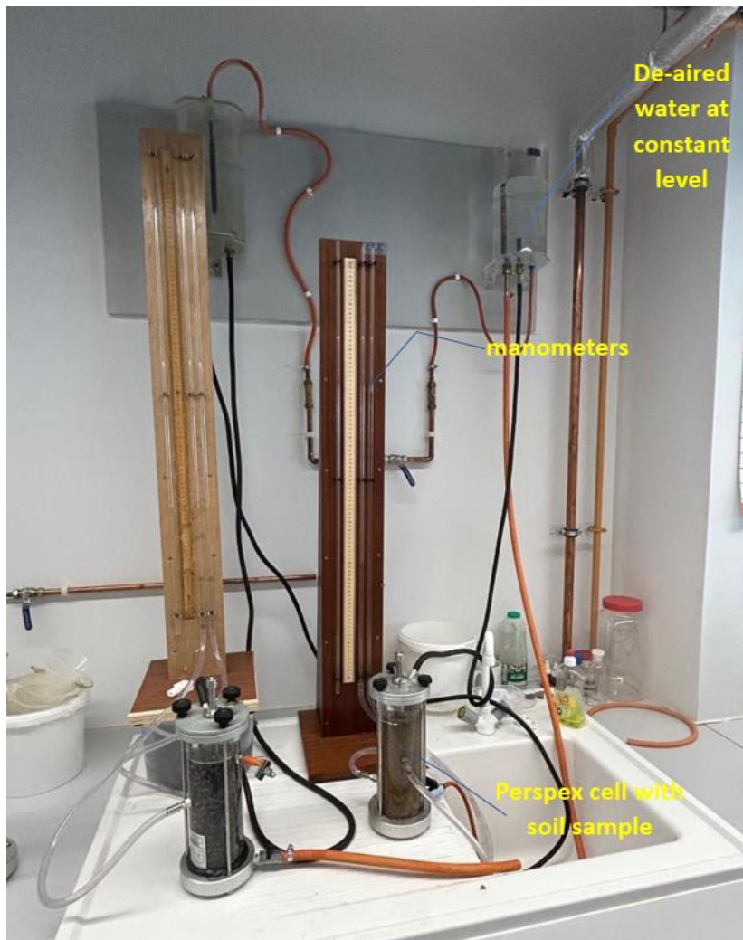
Photo of The Constant Head Apparatus set up.
