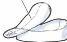
Screw on pouring spout provides control and re-close.
