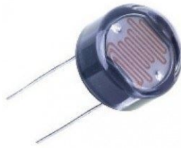
Figure 7. Leaded light dependent resistor (Spurr, 2014)
