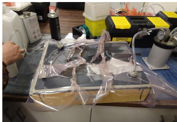
Figure 3 VARTM of carbon fibre bike seat (Chappell, 2017)
