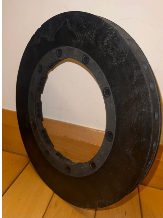
(Figure 7. Original brake rotor sample used for modelling)
