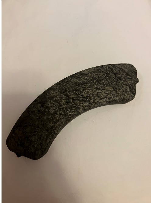
(Figure 9. Original brake pad sample used for modelling)
