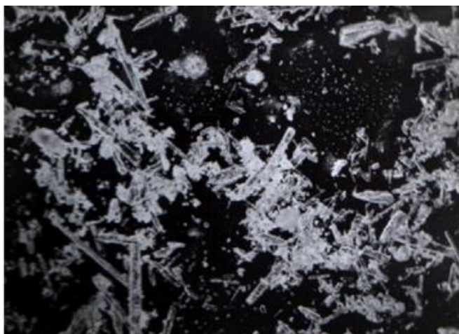
Figure 10-28 Basic lead styphnate (×80 magnification)
