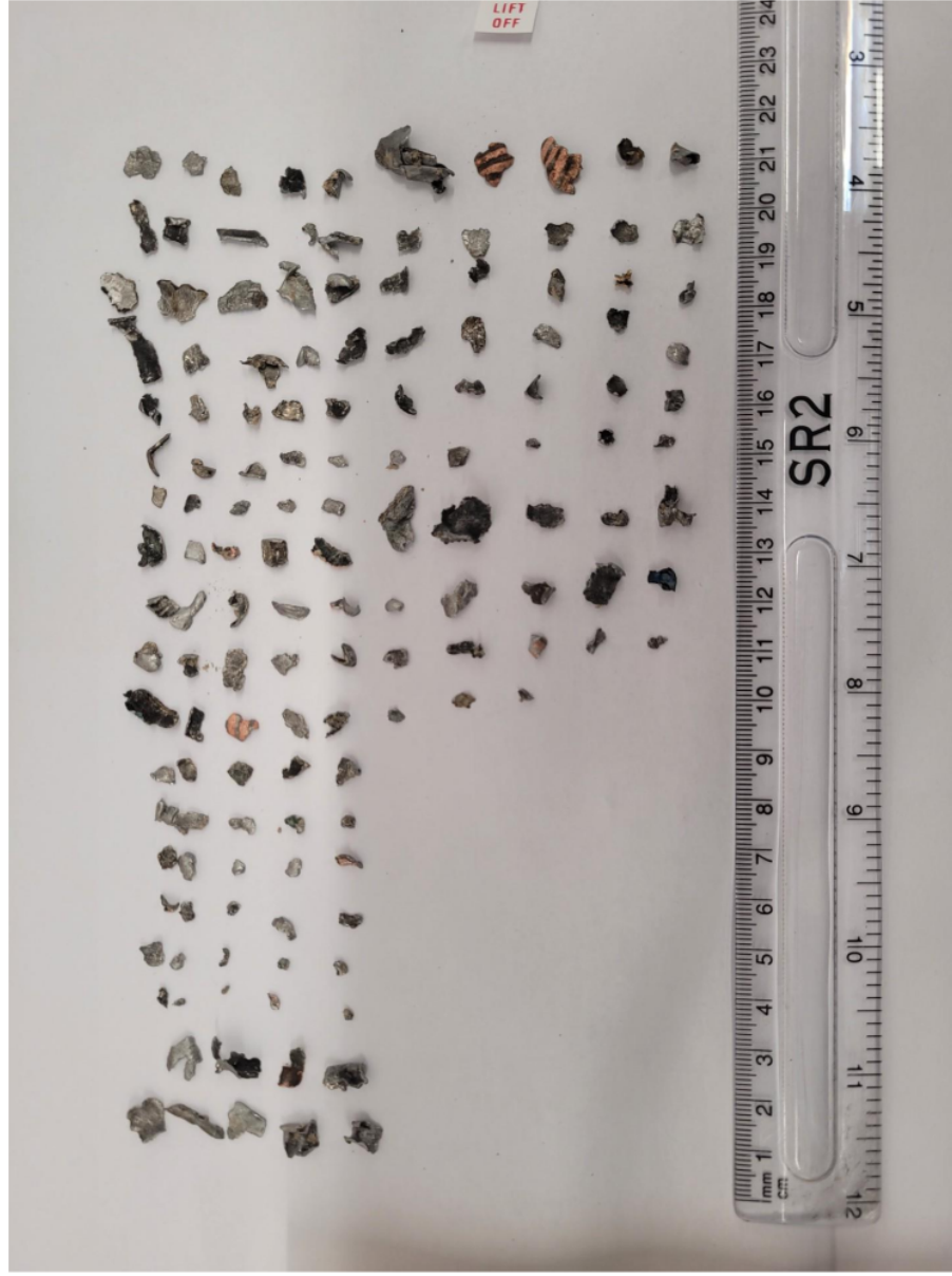
Figure 12: Fragmentation collected from the COTEC arena trial with a ruler included for scale.
