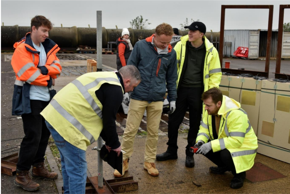
Figure 4: Distances of pressure gauges being checked with a laser range finder.
