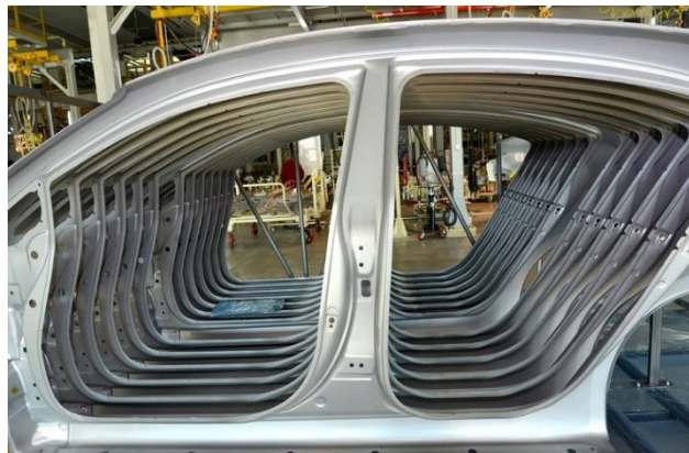
Figure 3: Pre pressed door sides from dies (Walendy, Sep 27, 2016)
