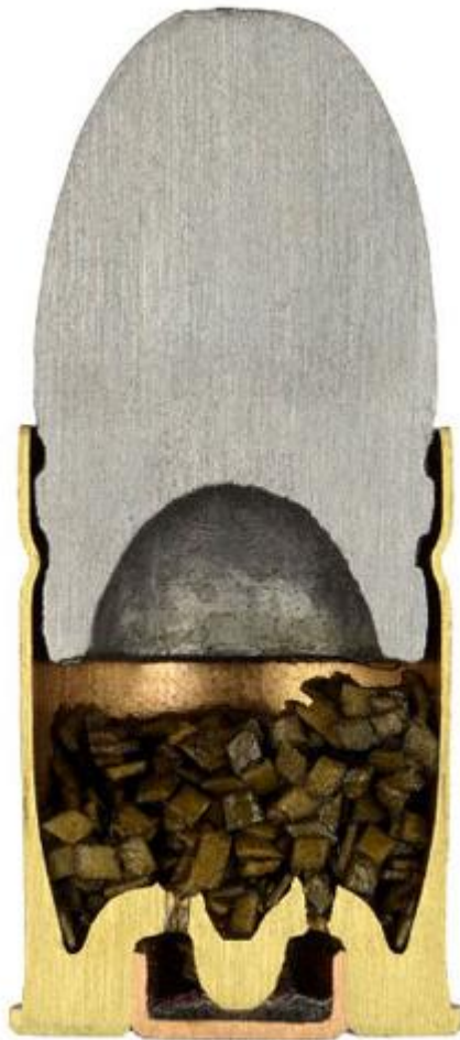
Figure 1 – Cross-section of 9x19mm bullet [1]
