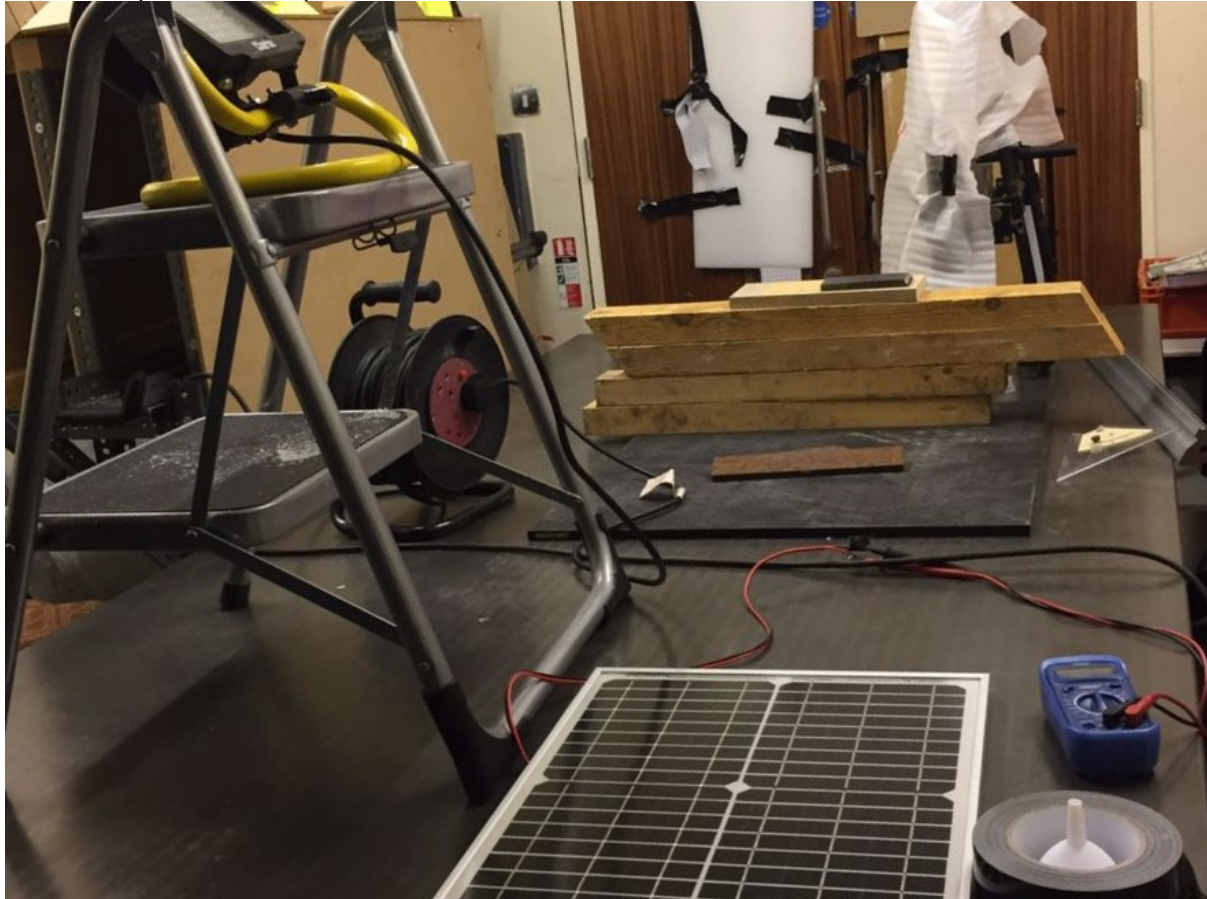
Figure 16: The Experimental Set-Up, Showing Panel. Light-Source. and Meter. Source: (Own Photo)
