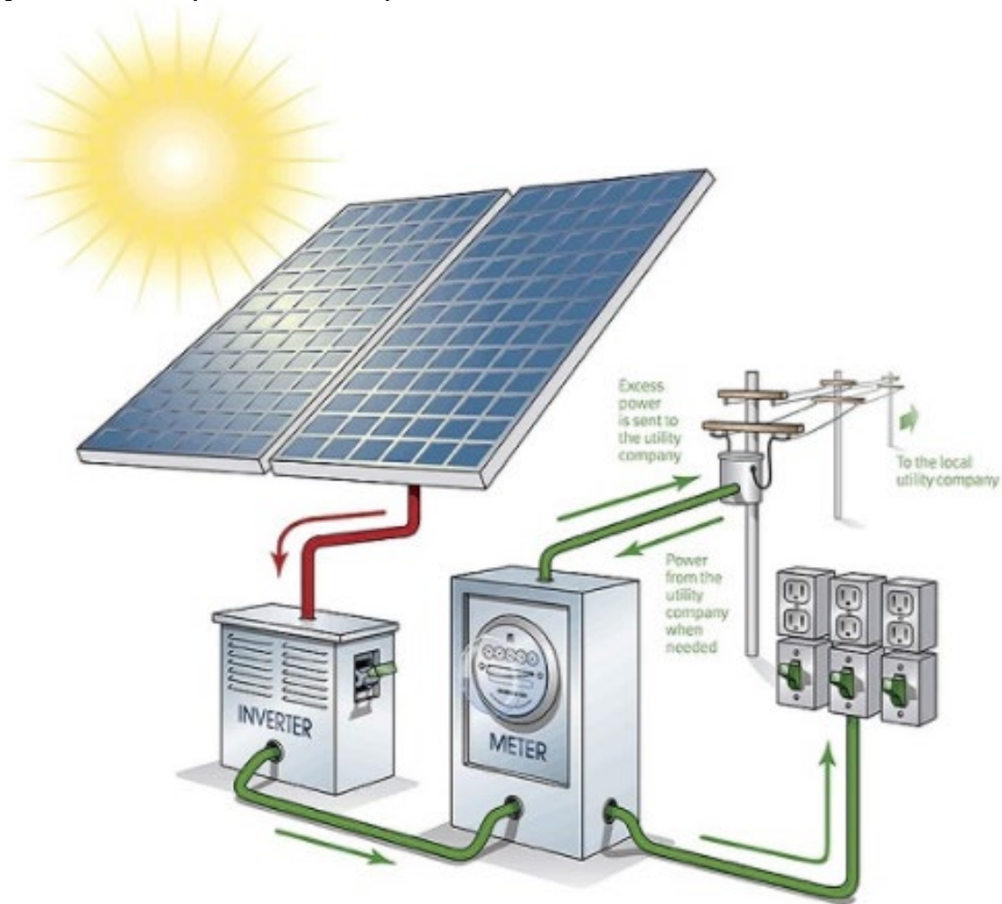
Figure 11: A Typical Small-Scale Solar Installation, Ideally Suited to this Project. Source: (Calsolar 2014)
