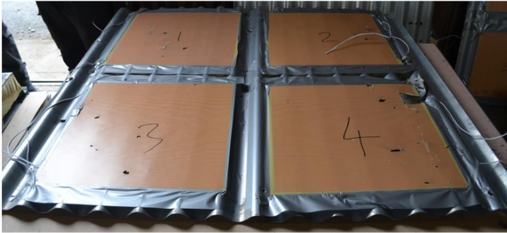
Figure 20- An unlabelled corrugated material post firing
