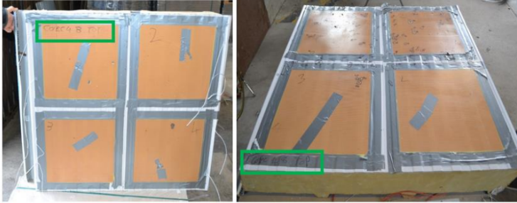
Figure 18- 2 different cladding sheets incorrectly labelled
