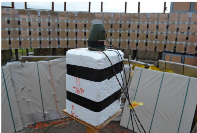
Figure 17- An inert representative mortar round positioned for firing 4
