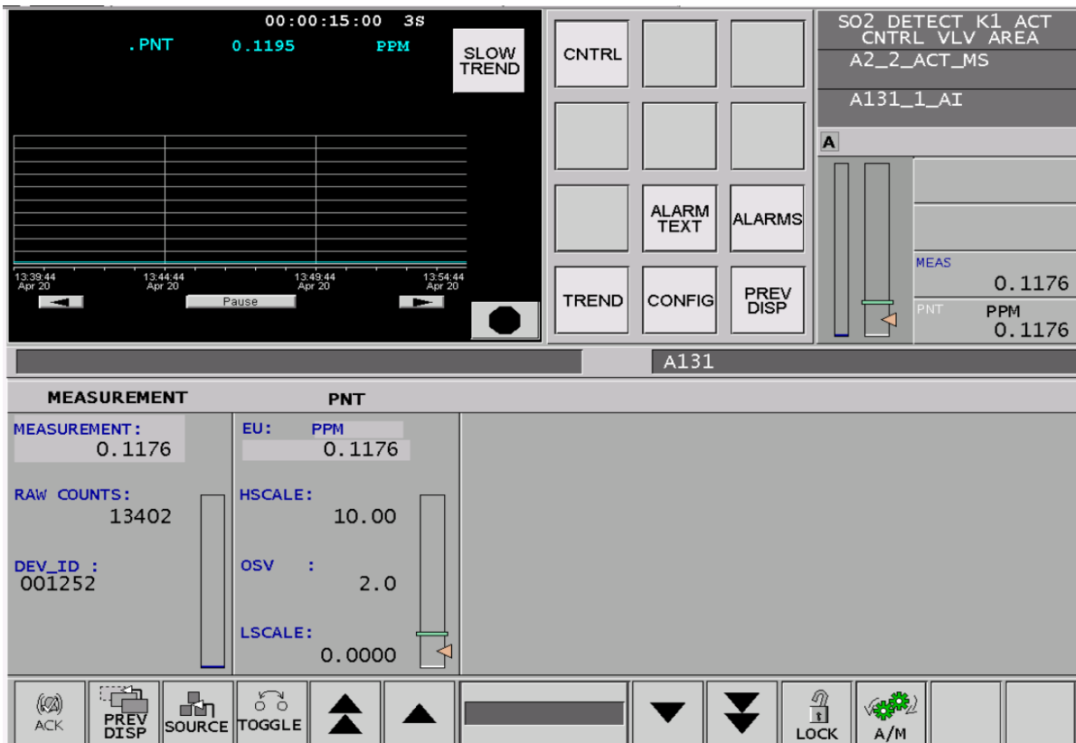
Figure.4: Individual Foxboro detector faceplate showing live ppm indication, alarm status, trend scaling, and operator navigation functionality.
