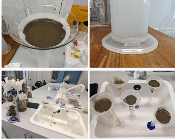
Figure 3.5: Manual filtration of water from spoil sample (Macfarlane, 2024e)
