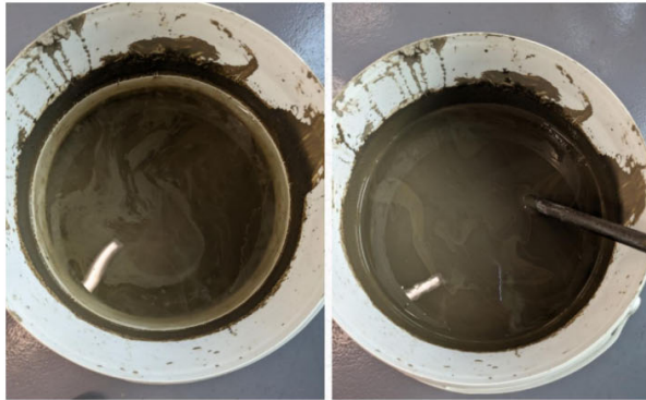
Figure 3.4: Water and spoil mixture after clay settling (L) and after manual mixing (R), (Macfarlane, 2024f)
