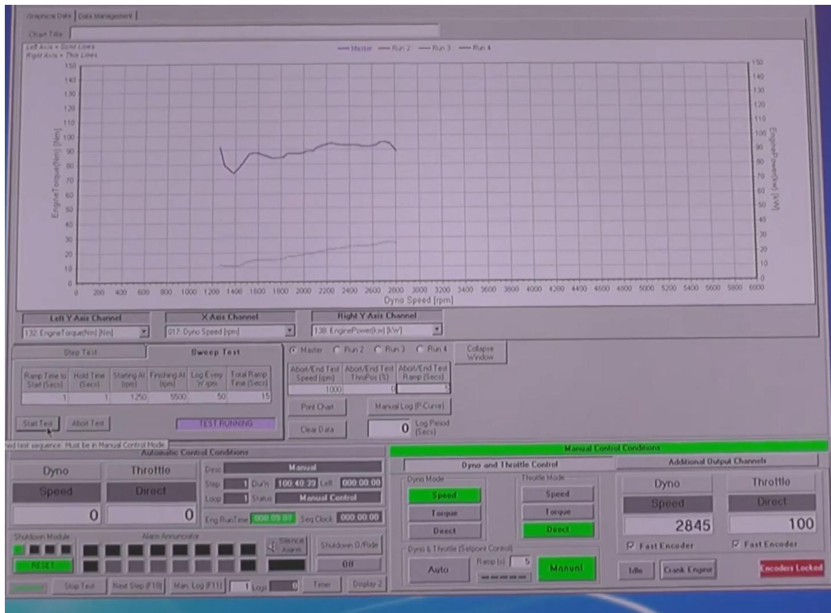
Figure 5 Computer Controls for Dynamometer (UWTSD WISA Workshops, 2020)
