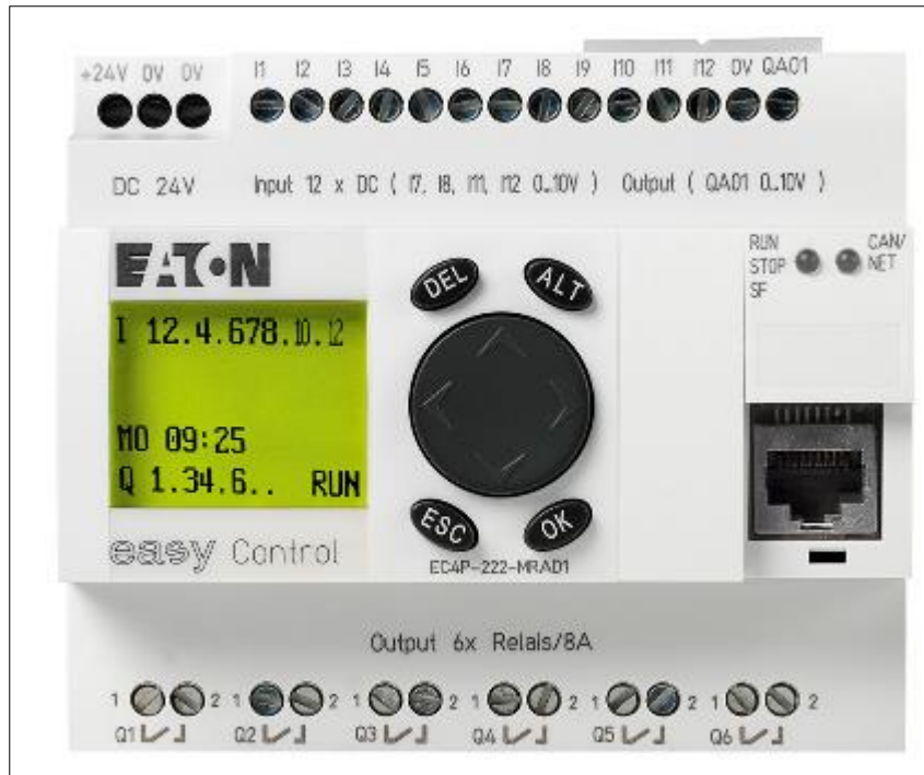
Figure 2: Compact PLC Source: Eaton company website
