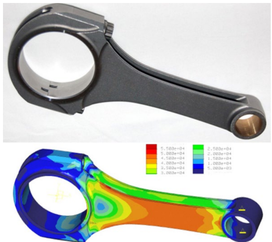
Figure 1- Showing Finite Element Analysis Carried out on a Con-Rod Assembly
