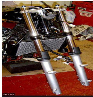
Figure 3- Showing a Motorcycles Yokes and Head-stock Assembly
