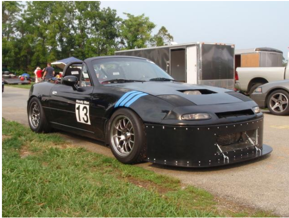
Figure 54 - An extreme air dam on a Mazda Miata (Occam's Racer, 2019)
