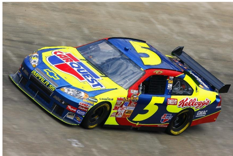
Figure 48 - An effective air dam-splitter combination on a NASCAR Generation 5 car (NASCAR Hall of Fame, 2026)
