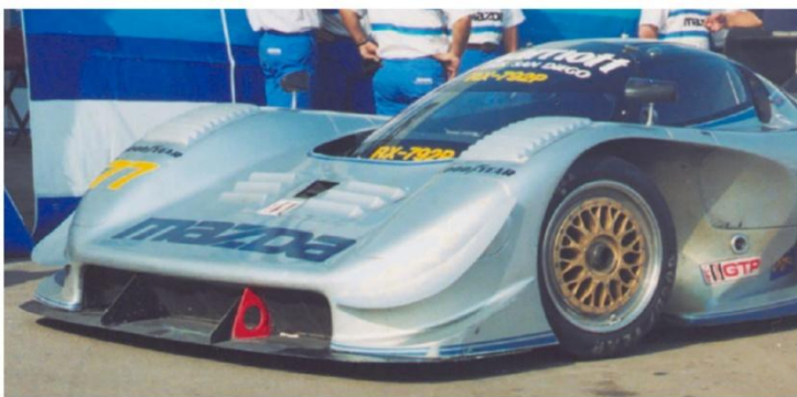
Figure 64 - A splitter as used on a Mazda RX-729P (Katz, J., 2019)
