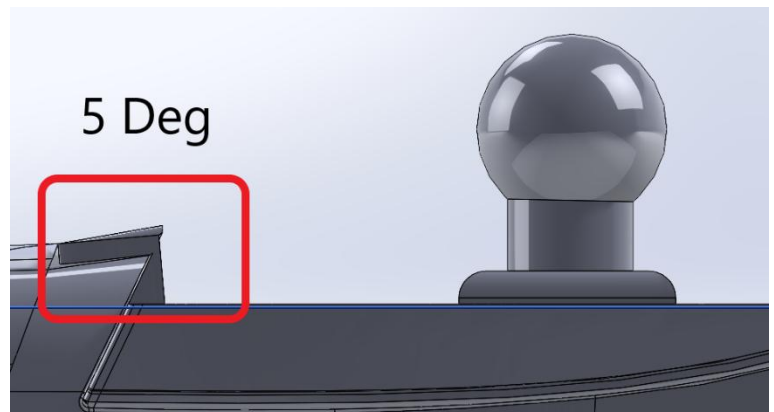
Figure 29 (5) Deg Air Deflector
