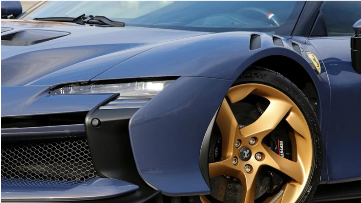
Wheel arch vents Rob Capaldi (2025)
