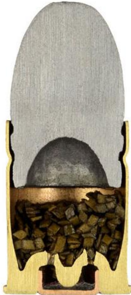
Figure 1 – Cross-section of 9x19mm bullet [1]
