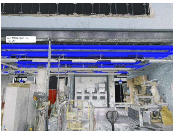
Fig. 13 – Laser scan using a Leica RTC360 (Revitzo 5 – ACBA 7002 Con. Tech.)
