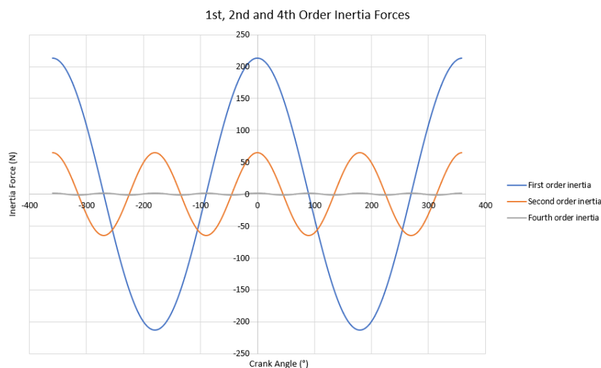
Figure 5 Different order Inertia forces.
