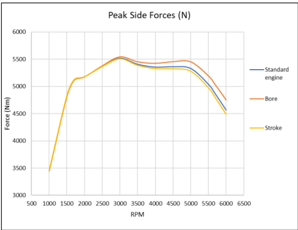
Figure 26 Peak side forces on each engine across the RPM range.
