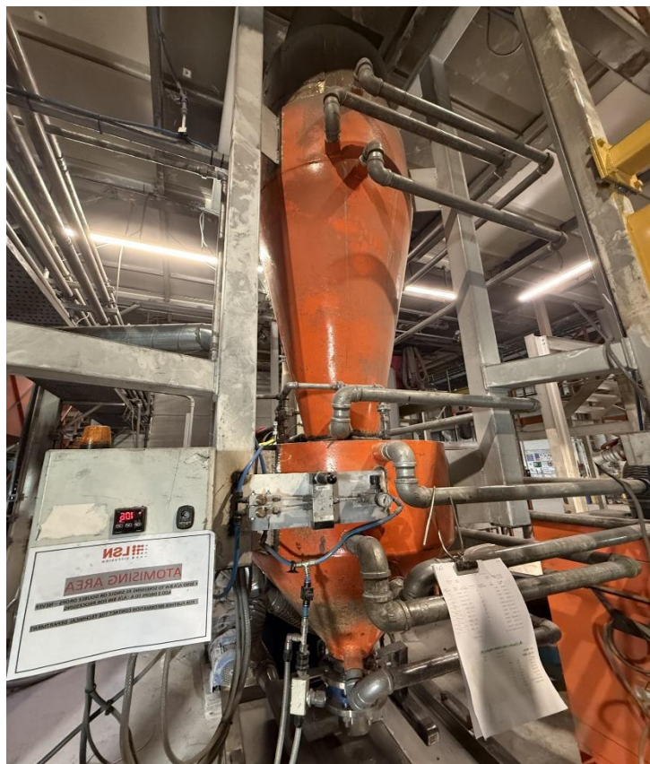
Figure 9 – Powder collection POD used to hold atomised metal powder and cooled with the aid of cooled water jackets.
