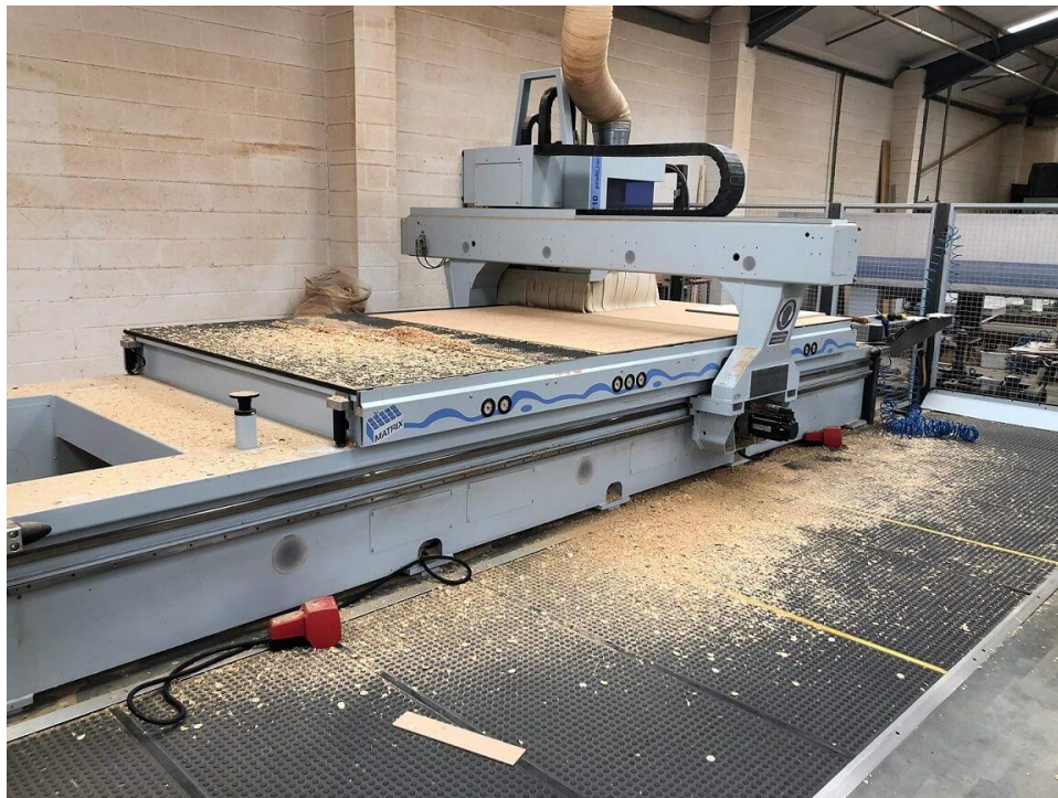
Figure 6. CNC mill producing MDF Laminate
