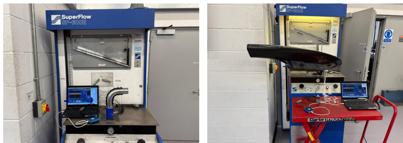
Flow-bench validation setup: 90° pipe test and pressure-tapped S2N+ airbox.
