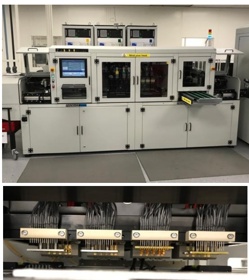
Figure 7: Electrical Test Machine (top) and Internal contact points (bottom) (Source: KSR & Thomas, 2017)
