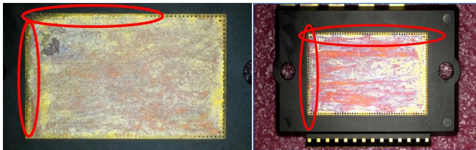
Figure 1: KSR power modules with defect DBC (left) and controlled DBC (right)
