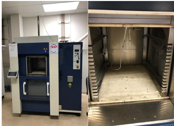
Figure 5: Thermal Shock Chamber (Source: KSR and Thomas, 2017)
