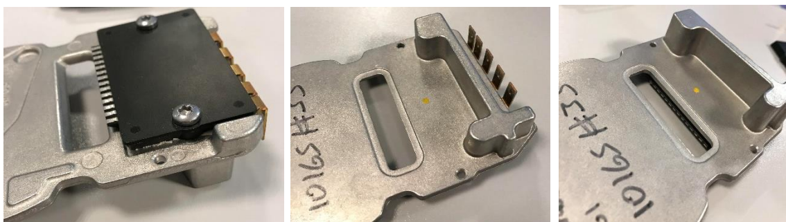
Figure 4: Power Module attached to customer's heatsink (Source: Thomas and KSR, 2018)
