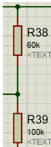
Figure11.2: Proteus circuit "Level-shift" gain controlled resistors
