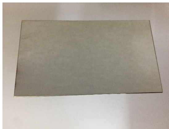
Figure 13: Initial state before corrosion and Class A (1% when the first stain appeared)
