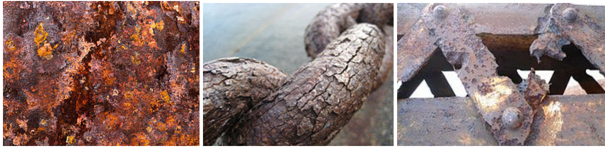
Figure 7: Heavy rust on iron/iron alloys (Gräfen, Horn, ESchlecker, & Schindler, 2000)
