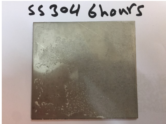
Figure 15: Class D (>25% corrosion level)
