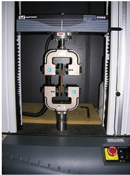
Figure 16: Tensile test machine and specimen set up
