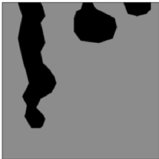
Figure 6: cross section of pitting corrosion (Gretchen, 2015)
