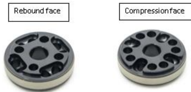
Figure 5-9 Showing the difference between rebound and compression side of the main piston
