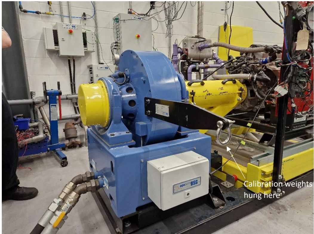
Figure 3: Calibration arm with loop for hanging weights.
