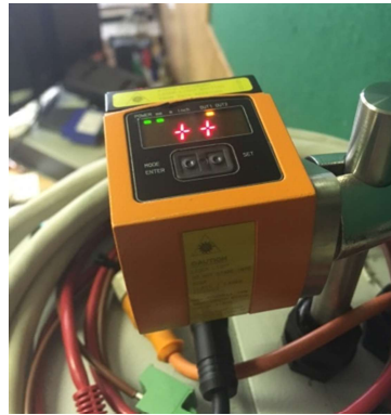
Figure 100 - Laser fault "Too much light"
