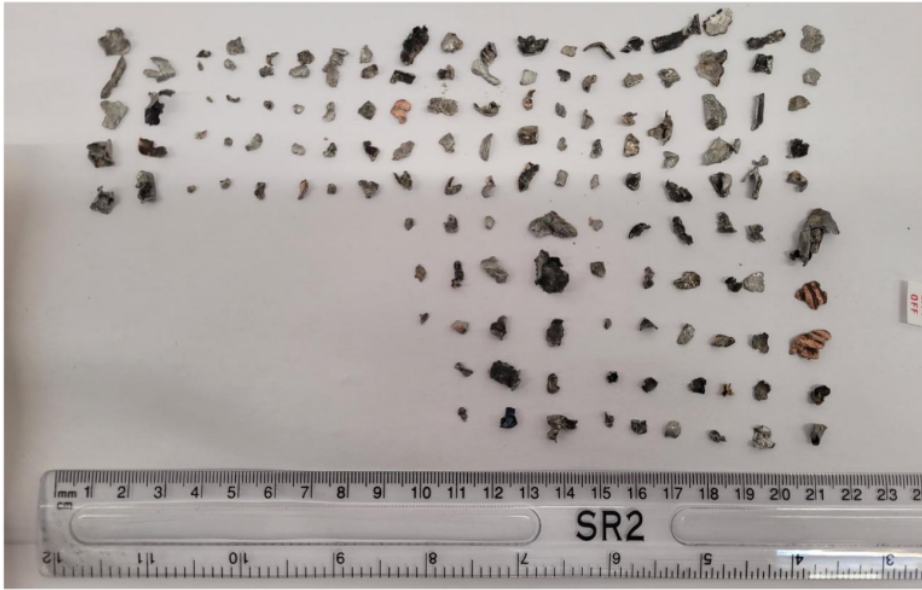
Figure 2: Fragmentation collected from strawboards.
