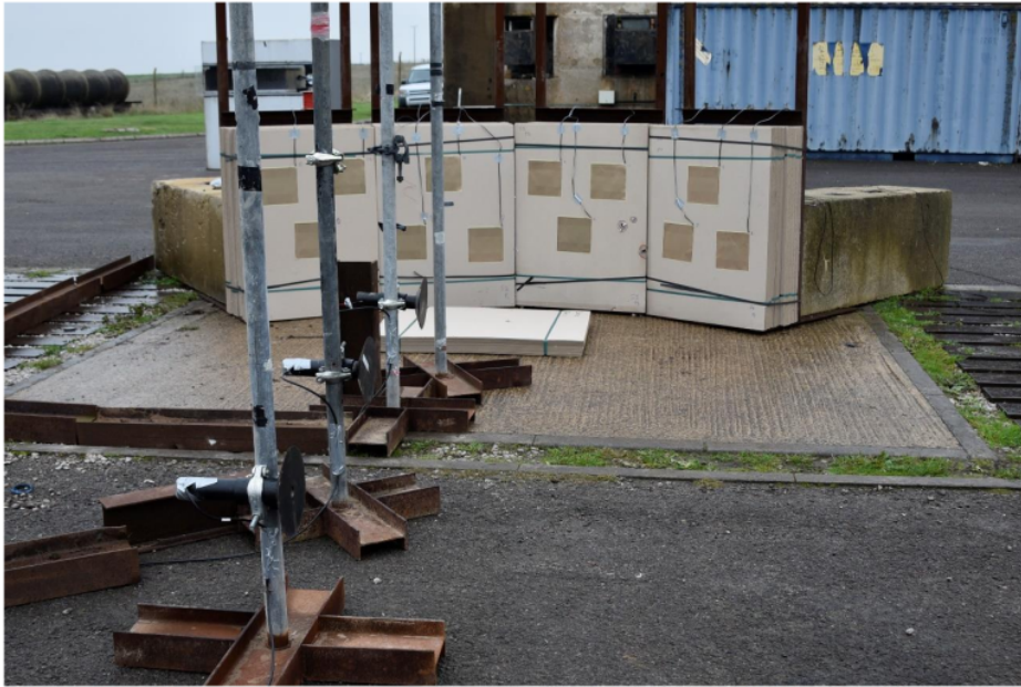
Figure 1: Arena setup for unknown munition, including Blast Overpressure (BOP) gauges, strawboards, and velocity foils.
