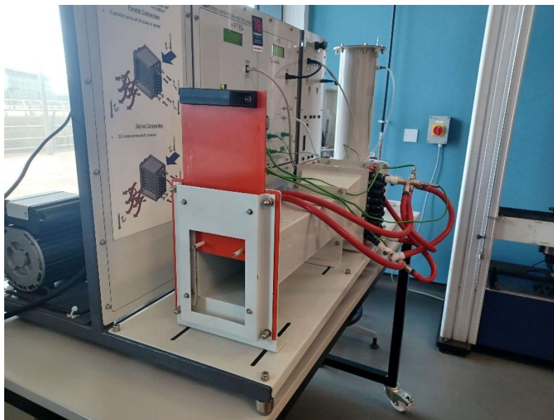
Figure 3: Airflow Control Hatch
