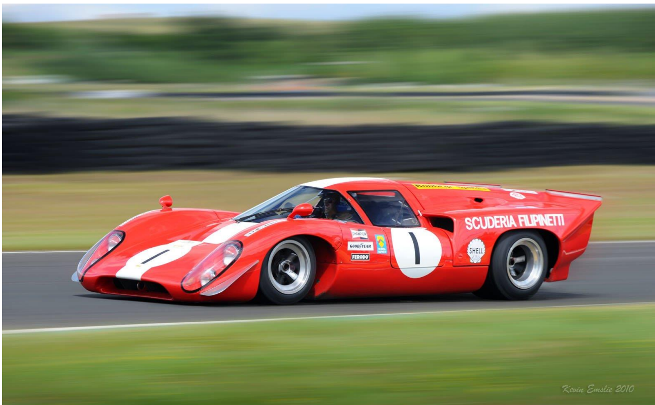
Figure 2 - Example of Rake Angle in a 1969 Lola T70 (Classic Drive Ltd, 2020)
