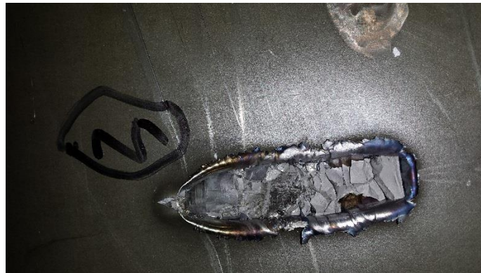
Figure 15 - Non-perforation, Front of Back Plate (12 mm plates separated by 3m)
