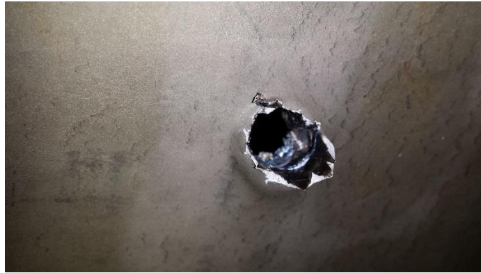
Figure 14- Exit Hole, Back Plate (12 mm plates separated by 2m)
