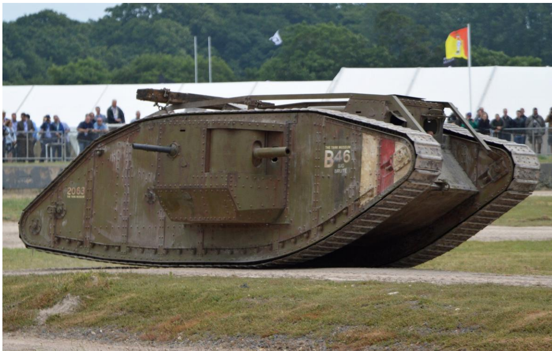
Figure 1: Mark IV British Tank from WW1 showing the rhomboidal caterpillar tracks, by Alan Wilson from Stilton, Peterborough, Cambs, UK, licensed under the Creative Commons Attribution-Share Alike 2.0 Generic license.
