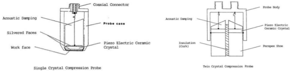
Figure 6 - Single and Twin Crystal UT Probes (HSE, 1994)
