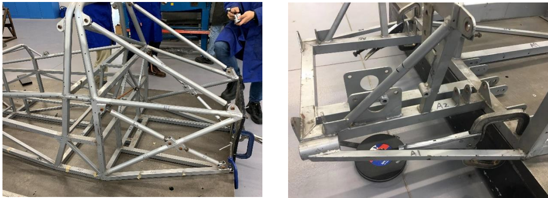
Figure 3-1 The fixing part of the vehicle structure
