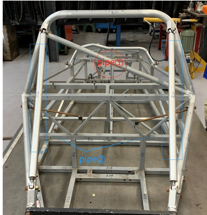
Figure 3-27 Tubes removed in different sets of the test
