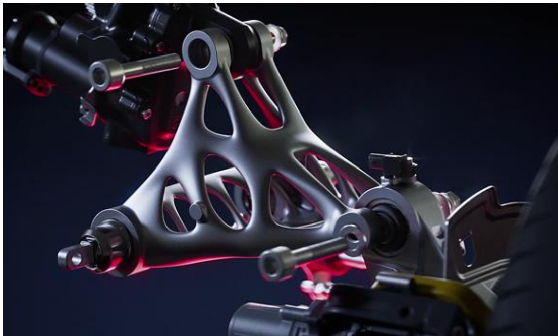
Figure 19-Ferrari F80 AM design control arm. (AM, 2025)
